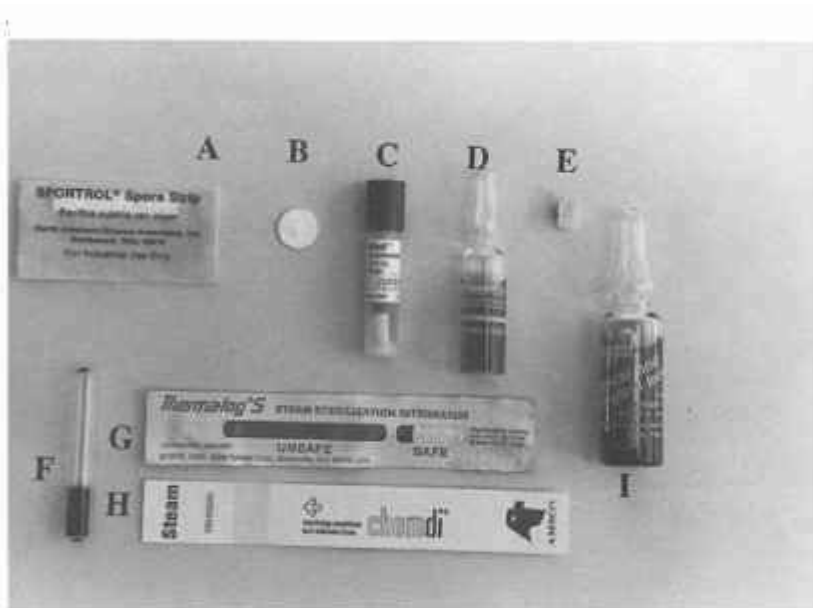
Fig. 23.1 Examples of biological and chemical indicators used for monitoring sterilization processes. (A and B) A spore strip (in a glassine envelope) and a spore disc, respectively; the spores are dried onto absorbent paper or fabric. (C) Attest™ indicator comprising a plastic vial containing a spore strip together with a sealed glass ampoule of culture medium; the ampoule is crushed after exposure and the medium immerses the strip. (D) Chemsport™ indicator in which bacterial spores are suspended in culture medium; the horizontal band on the ampoule also darkens on autoclaving to enable steam-exposed and non-exposed ampoules to be distinguished. (E) Plastic carrier with dried Bacillus stearothermophilus spores designed for monitoring low-temperature steam and formaldehyde cycles. (F) Browne's tube™; the liquid within the tube changes colour on heat exposure. (G) Thermalog™ strip in which a blue dye progresses from left to right during heat exposure. (H) Chemdi™ displays colour change in arrowed section of the strip after heating. (I) Chemsport™ which is a combined chemical and biological indicator; the ampoule contains a spore suspension in culture medium together with a second, smaller ampoule which contains a chemical indicator.
