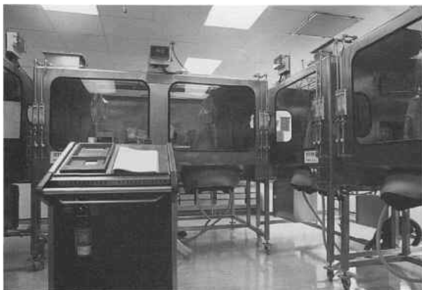
Fig. 23.2 Isolators used for sterility testing. The operator works within the hood which is suspended inside the cubicle; the hydrogen peroxide generator which is used to sterilize the isolators is shown in the left foreground. (Courtesy of SmithKline Beecham Pharmaceuticals.)
